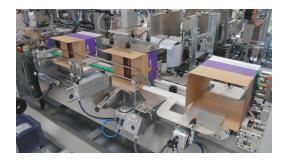
Sidel has launched a new Cermex WB47 case packer, expanding its WB wrap-around range to handle not only the wrap-around blank family, but also American cases (RSC and HSC). Additionally, the upgraded WB platform ensures enhanced flexibility with shorter changeover times. In 45 years, Sidel has installed more than 8,000 packers, including 1,000 wrap-around machines. More than 130 units of the best-seller Cermex WB46 and the new Cermex WB47 have already been manufactured in four years.
